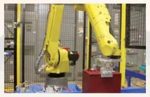
**Advanced Robotics** Advanced robotics are used throughout Trojan's manufacturing plant to ensure a higher level of product consistency and quality. Robotics streamline our battery production and improve our manufacturing lead time.
